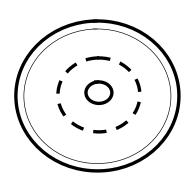
CUT OR TEAR ON THE OIL SIDE OF THE DIAPHRAGM THAT CORRESPONDS TO THE DIAMETER OF THE PISTON:
