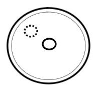
CUT OR TEAR ON THE OIL SIDE OF THE DIAPHRAGM THAT DOES NOT COR RESPOND TO THE DIAMETER OF THE DISC OR PISTON:
