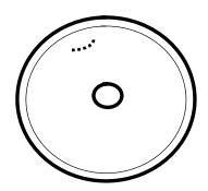
CUT OR TEAR ON THE CHEMICAL SIDE OF THE DIAPHRAGM THAT CORRE SPONDS TO ONE OF THE VALVE OPENINGS ON THE UNDERSIDE OF THE PUMP HEAD:
